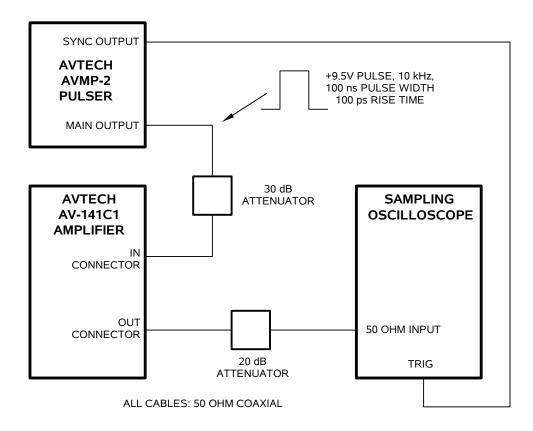
The recommended test set-up is shown above.
